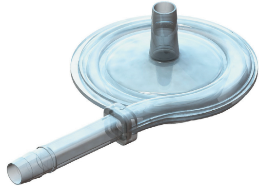
Fig. 1. Reconstructed 3D model of the RotaFlow pump (Maquet, Germany)
