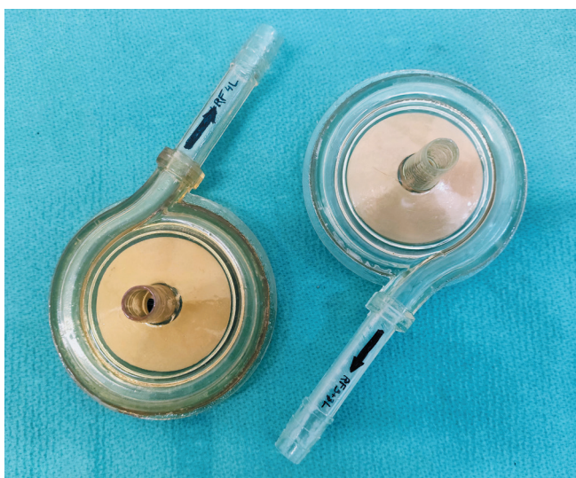
Fig. 3. Experimental photopolymer pump models with the original and modified rotor designs
