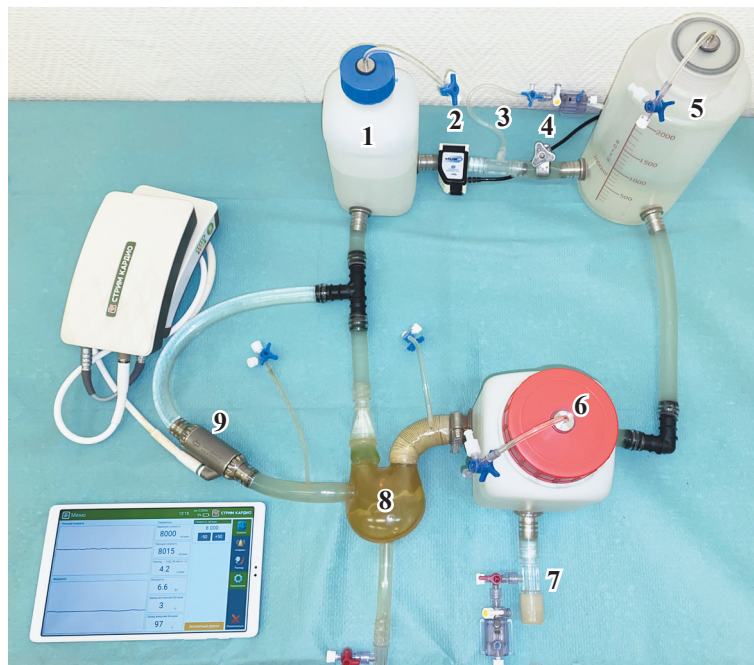
Fig. 3. Mock circulation loop. 1, arterial reservoir; 2, aortic flow sensor; 3, arterial pressure measurement sensor; 4, systemic hydraulic resistance; 5, venous reservoir; 6, reservoir simulating the “pulmonary veins, left atrium” system; 7, atrial pressure measurement sensor; 8, cardiac ventricle simulator simulating the left ventricle of the heart during a left ventricular bypass; 9, test pump
