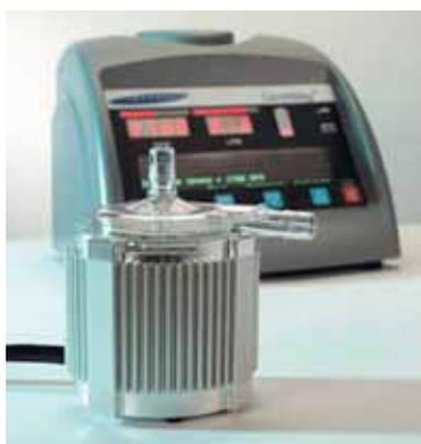
Fig. 5. CentriMag drive system
