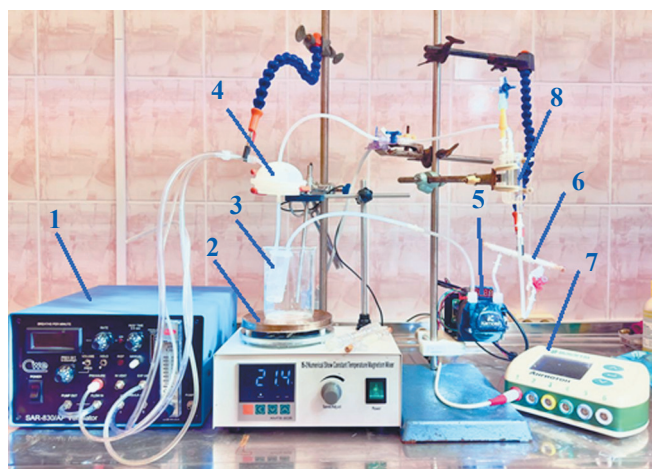
Fig. 2. The developed bench for normothermic machine perfusion of lungs in small animals (1, ventilator; 2, heating device; 3, sealed container; 4, developed container for donor lungs; 5, roller (peristaltic) pump; 6, developed low priming volume membrane oxygenator; 7, pressure measuring apparatus; 8, bubble filter)
