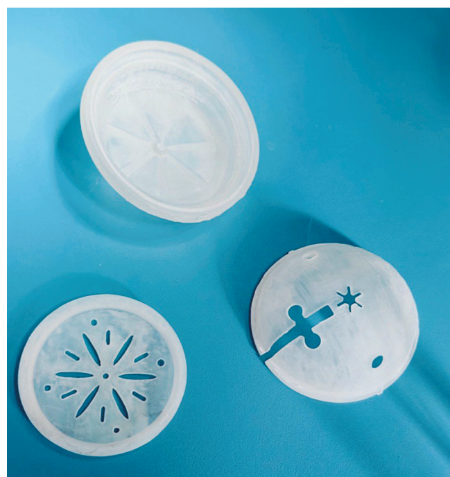
Fig. 4. Manufactured parts of the container for placing donor lungs of small animals
