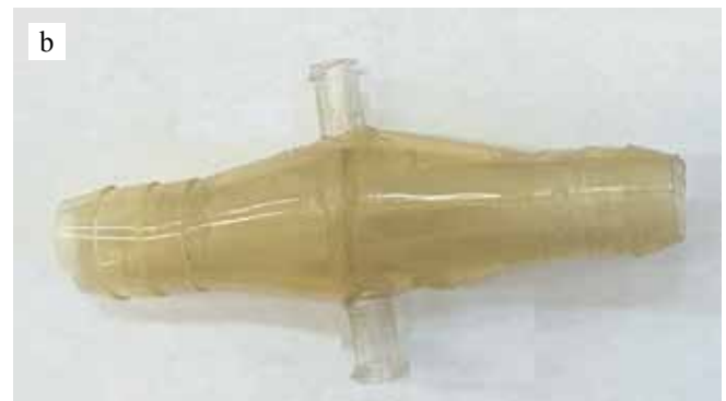
Fig. 1. a, schematic diagram of pulsator (1, hull; 2, elastic tube; 3, holes; 4, air cavity; 5, flow path); b, external view of pulsator
