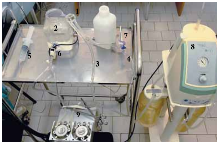
Fig. 7. Hydrodynamic bench. 1, cannula; 2, cardiomy tank; 3, air channel; 4, liquid channel; 5, air supply device; 6, flow measurement / microbubble counting sensor; 7, vacuum measurement sensor; 8, vacuum suction tank; 9, roller pump
