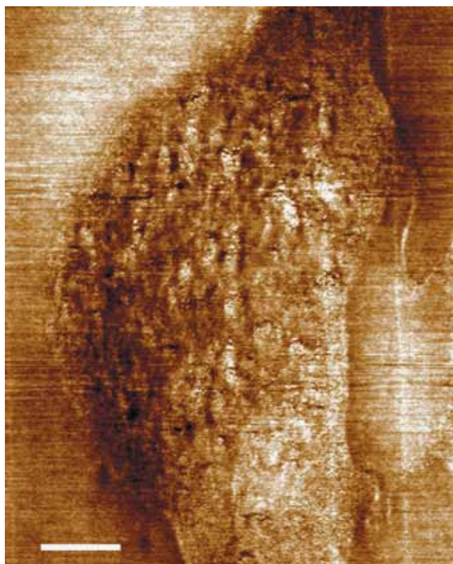
Fig. 4. SPM image of the topography of a cross-section of the silk fibroin-based film scaffold with adhered liver cell: scan size 7.0 \times 6.0 \mu\text{m} , height variation range 20 nm, scale bar 1 \mu\text{m}
