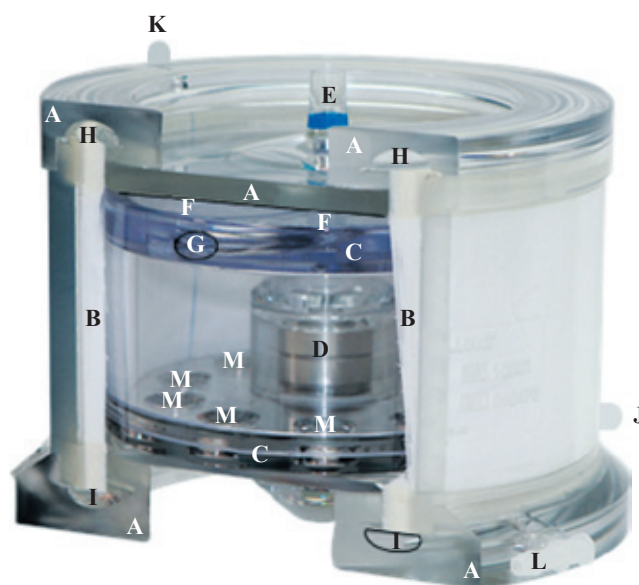
Fig. 2. Hemolung Respiratory Assist System gas exchange cartridge (frontal cut): A – gas exchange cartridge housing; B – gas exchange polypropylene membrane bundle; C – integrated rotating barrel; D – bearings; E – upper pipe connector; F – spare space between housing and barrel; G – channel inside the barrel; H – inflow gas channel; I – outflow gas channel; J – bottom pipe connector; K, L – pipe connectors; M – integrated magnets.
