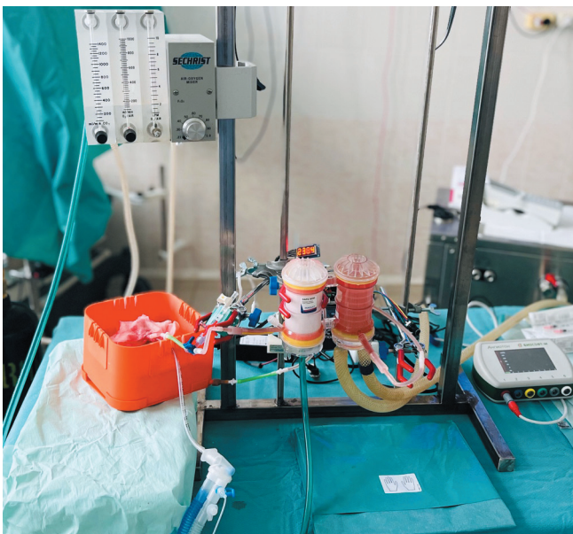
Fig. 2. Perfusion circuit setup for normothermic EVLP
