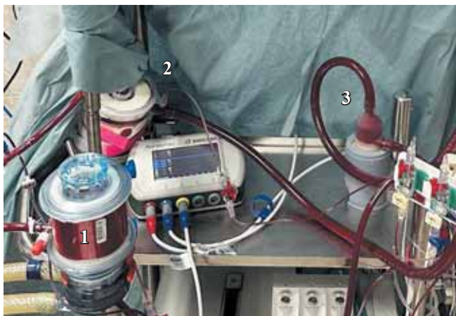
Fig. 5. Evaluation of oxygenating properties and hemolysis in ECMO mode (1, LivaNova oxygenator (INSPIRE, USA); 2, deoxygenator; 3, developed centrifugal pump)
