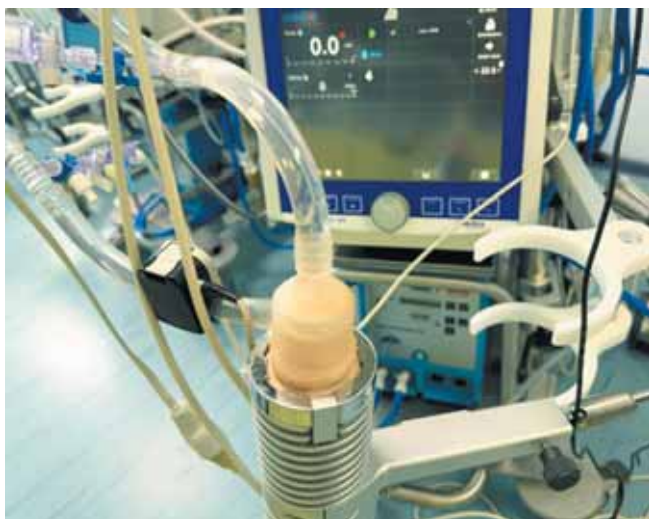
Fig. 4. Evaluation of the HCC of the fabricated centrifugal pump head
