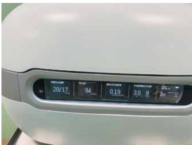
Fig. 4. External view and baseline kidney perfusion parameters in the LifePort Kidney Transporter
