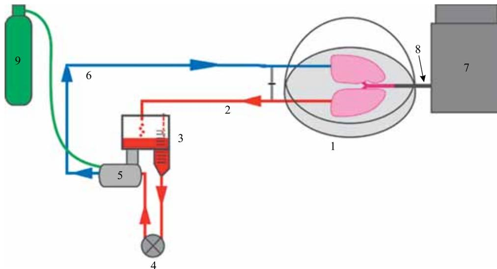
Fig. 1. Schematic layout of perfusion circuit. 1, Open organ chamber; 2, left atrial line; 3, cardiotomy reservoir; 4, centrifugal pump; 5, oxygenator; 6, venous line to the pulmonary artery; 7, ventilator; 8, air line; 9, balloon with deoxygenating mixture connected to oxygenator
