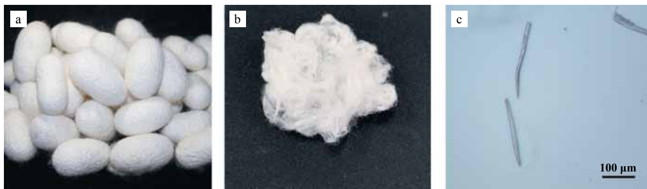
Fig. 1. Fabrication of fiber microcarriers. a) Bombyx mori silkworm cocoons; b) sericin-free silk fibroin; c) fiber microcarriers. Scale bar 100 \mu\text{m}
