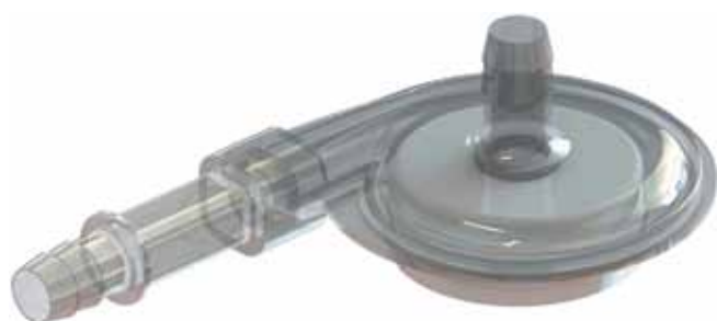
Fig. 1. Calculation model of the channel centrifugal pump
