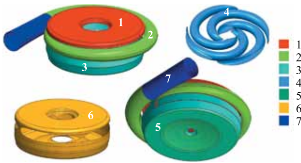
Fig. 2. Pump areas for investigation. 1, upper zone; 2, spiral outlet; 3, lateral zone; 4, channel zone; 5, lower zone; 6, impeller zone; 7, diffuser zone
