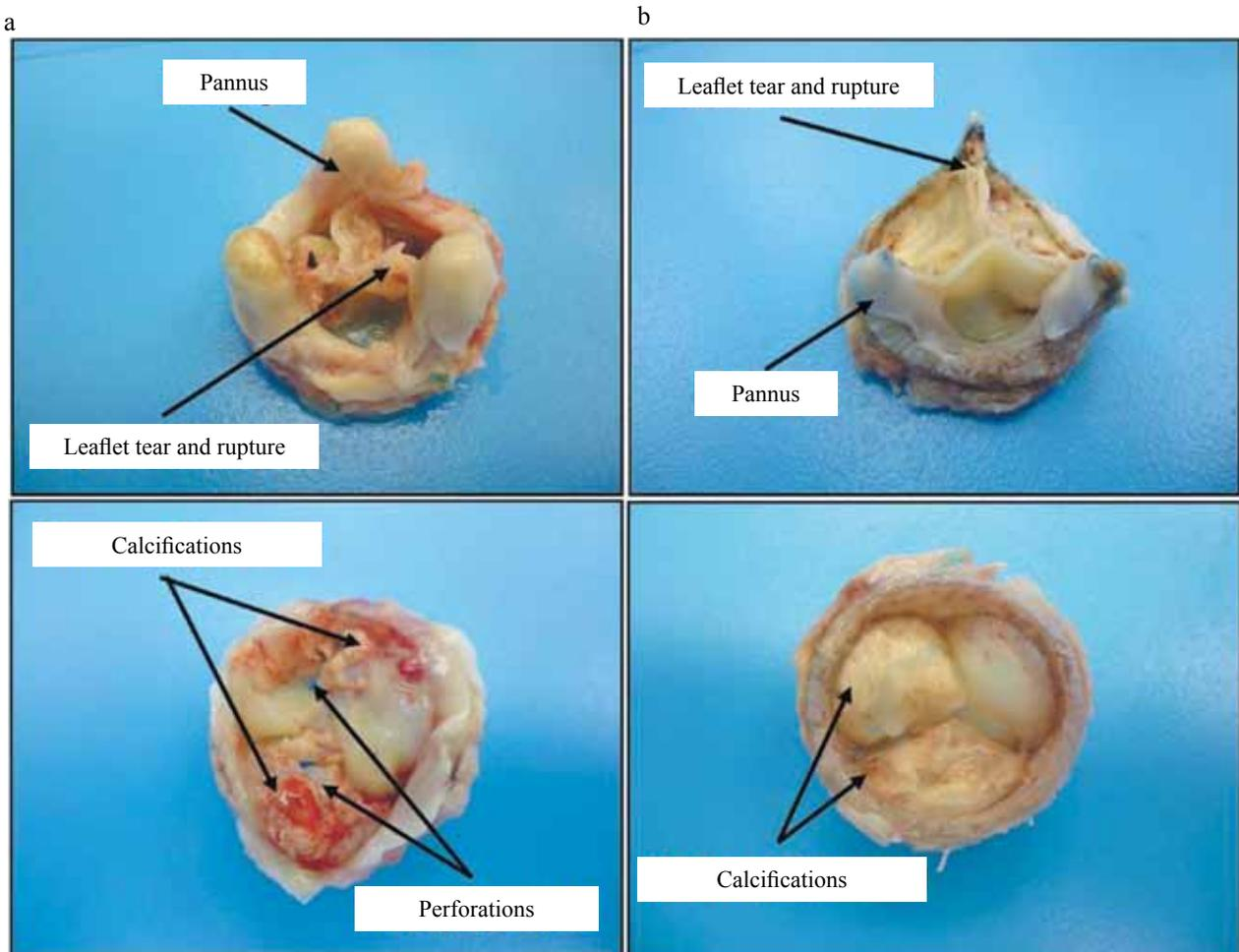
Fig. 1. Heart valve bioprostheses removed due to dysfunction: a – xenoaortic prosthesis (PeriCor); b – xenopericardial prosthesis (UniLine); Upper and lower rows – view from the outflow and inflow side, respectively
