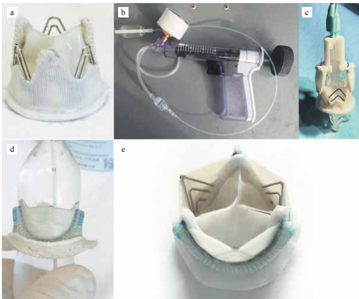
Fig. 1. Material and methods: a – design of the developed prosthesis; b – a delivery system comprising a balloon catheter and a high pressure syringe-defuser; c – re-implantation system with holder; d – the result of “valve-in-valve” implantation immediately after balloon dilation; e – the same, in the final state before the hydrodynamic study
