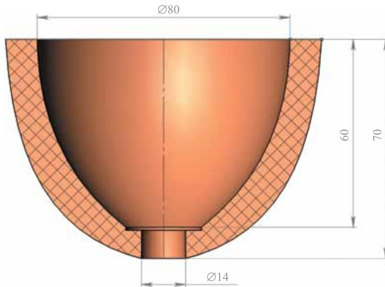
Fig 4. The geometry of the ventricle model
