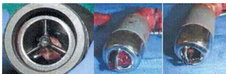
Fig 2. Pump inlet thrombosis
