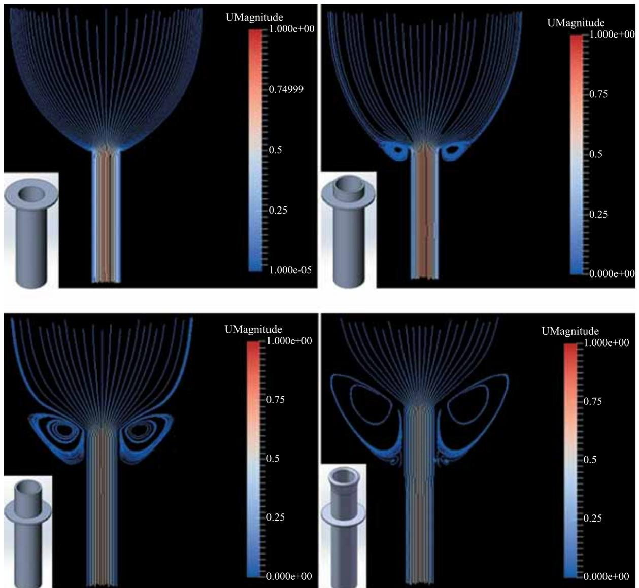
Fig 5. Results of modeling blunt tip cannulas
